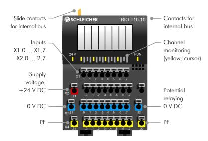
The RIO T10-10 expert module allows temperature measuring in the important industrial range of -100  $^{\circ}$ C to +450  $^{\circ}$ C. It provides four inputs for standard PT100 and PT1000 platinum shunts. Using the sensor resistance the module automatically recognizes the type of sensor, so external configuring is unnecessary. The choice of 2-wire, 3-wire or 4-wire connection systems allows precision to be matched to requirements.
